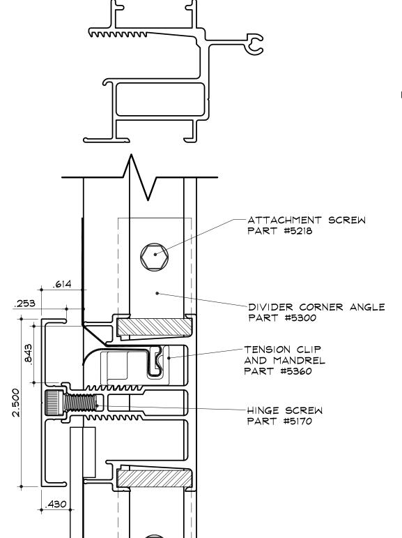
DRILL %" HOLE EVERY 36" ON CENTER FOR INERTION OF HINGE SCREW TO FASTEN COVER.
